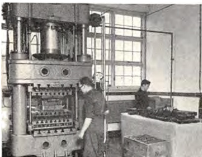
Moderne hydraulisk Presse, Tryk: 300,000 kg.
