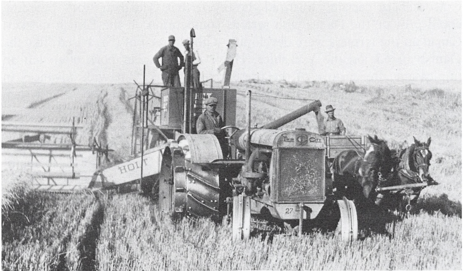
A combine for cutting and threshing in a single operation.
